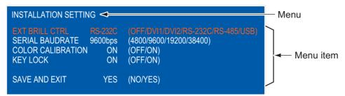
For ECDIS (FEA-2107) or chart radar (FCR-21x7), no adjustment is necessary. Keep this equipment in the default settings.
